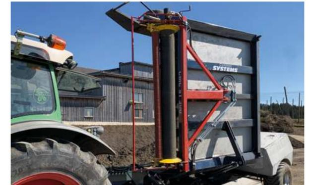
Every composting plant operator longs for not having to handle the compost protection fleece by hand. With this simple additional device, the fleece is simply left lying on the pile during the turning process and clamped to the guide roller, and in this way the fleece is simply pulled underneath. It's important that the fleece is guided high enough during the turning process so that the gas exchange is not impaired and the heat can also escape well from the core of the pile.
