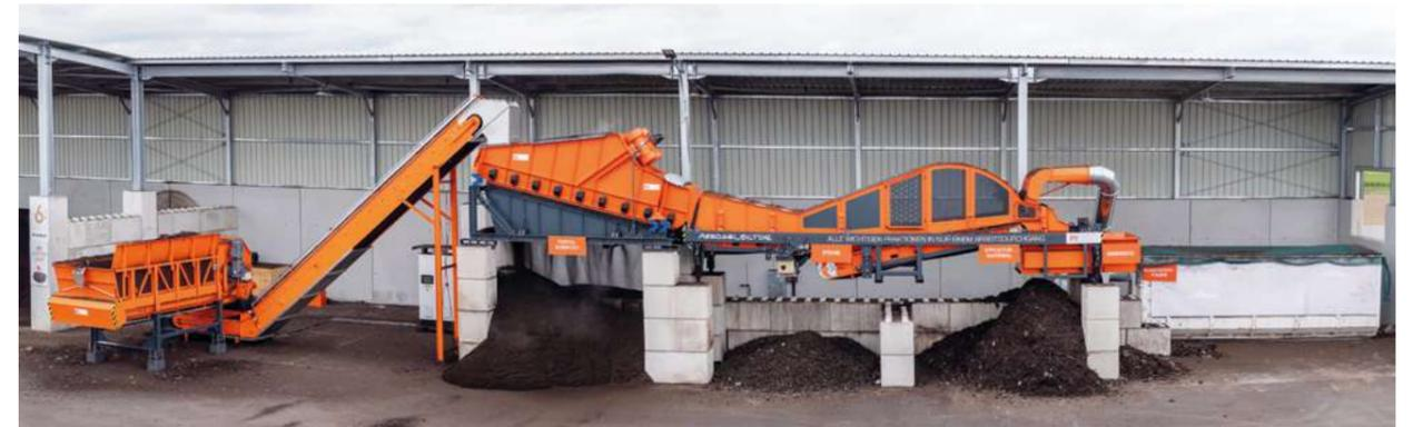
A combined screening unit with impurity removal for the screen overflow including air classifier, stone trap and magnetic separator.
