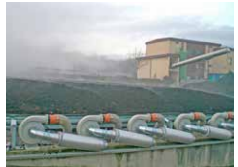
The "COMPOnent" aeration system was installed on the first composting plant in Austria in 1997. Today an annual volume of over 160,000 tons of sewage sludge is composted throughout Austria on 15 composting plants.
