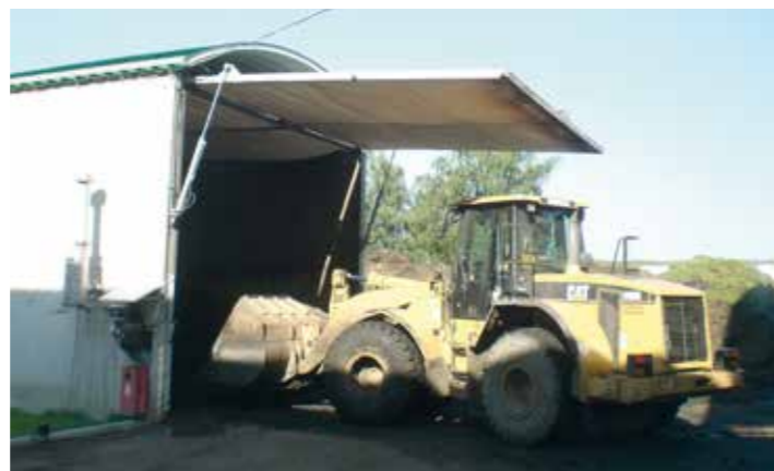
Loading and unloading the box without removing the membrane
