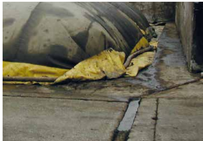
Leachate can flow out from the sides of the membrane. This water can in certain circumstances cause higher odour emissions than the windrow itself!
