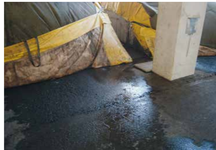
Leachate can flow out from the sides of the membrane. This water can in certain circumstances cause higher odour emissions than the windrow itself!
