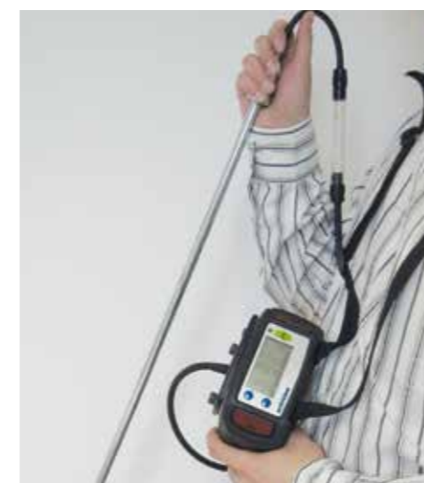
This windrow gas meter measures up to 5 different gases at the same time.
