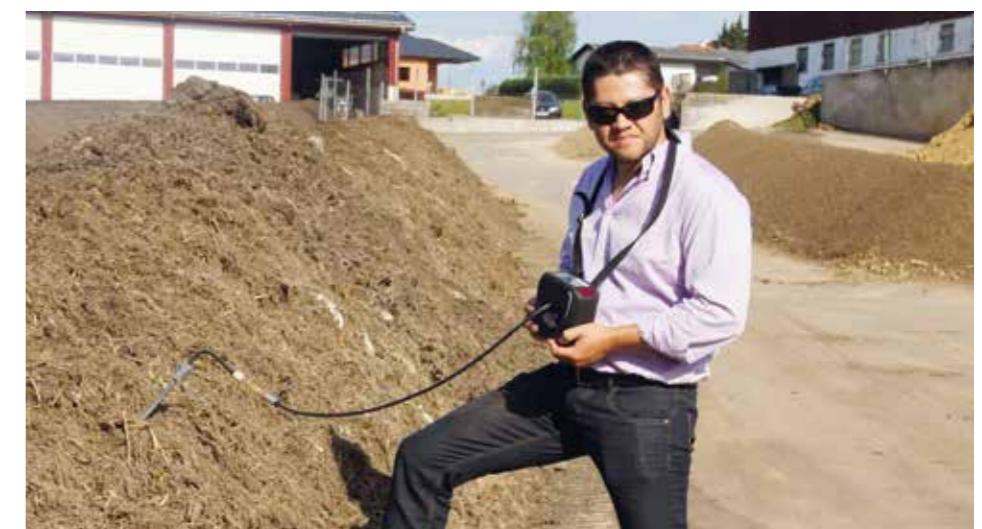
This windrow gas meter measures up to 5 different gases at the same time.
